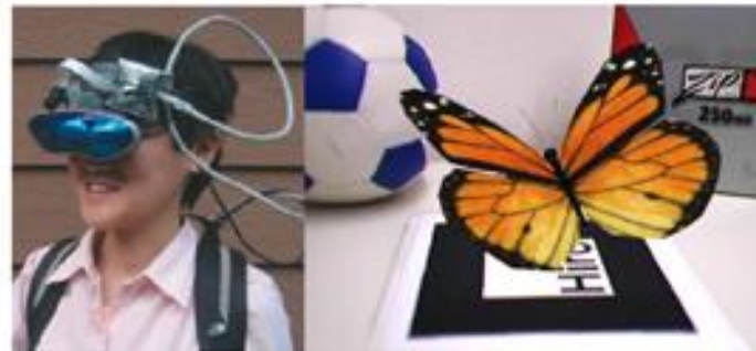
See-through AR: the butterfly is computer-generated, and everything else is real (Fischer, Bartz & Straßer, 2006; Kölsch, Bane, Höllerer, & Turk, 2006).
