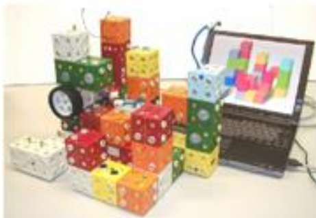
Using physical objects to create a virtual model (Ichida, Itoh, & Kitamura, 2004). As a user adds a physical 'ActiveCube' to the construction, the equivalent virtual model is automatically updated.
