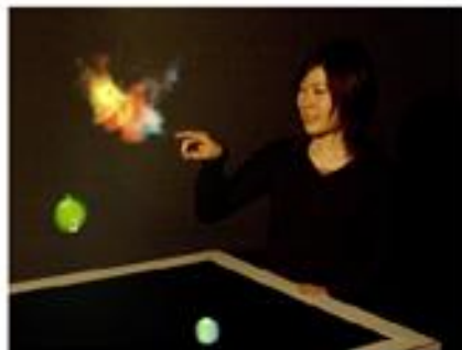
The 'Bubble Cosmos' – 'Emerging Technology' at SIGGRAPH'06. The paths of the smoke-filled bubbles are tracked, and an image is projected into them as they rise.
