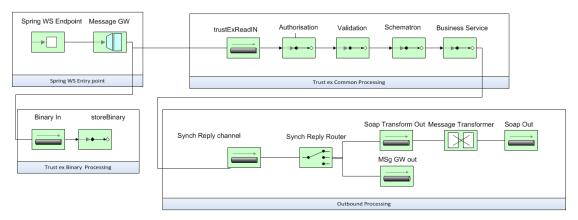
The *Store Document Wrapper* web service interface uses MTOM to optimize the size of the transferred encoded binary size and HTTP chunking to allow the streaming of the binary file to the disk.
