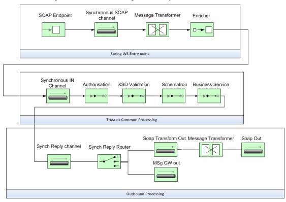
The platform offers two entry points to provide synchronous service. They are both SOAP based but use different web services implementation.
