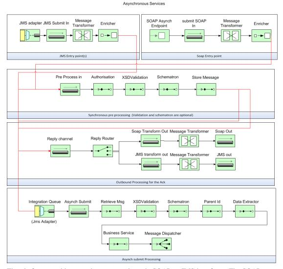
The platform provides asynchronous services via SOAP or JMS interfaces. The SOAP entry point for asynchronous services uses the same components as the one for synchronous services.
