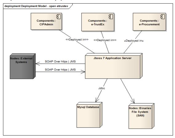
It is important to note that not all physical nodes are represented on this diagram. Indeed Database Servers and Application Servers could be duplicated for scalability and availability reasons. Furthermore, security mechanisms like firewalls are not shown.
